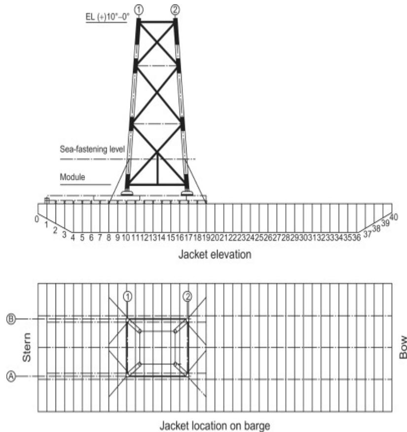
Figure 5.43. Jacket sea fastening during transportation.
