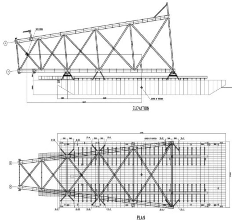
Figure 8.92. Structure model located on the barge.
