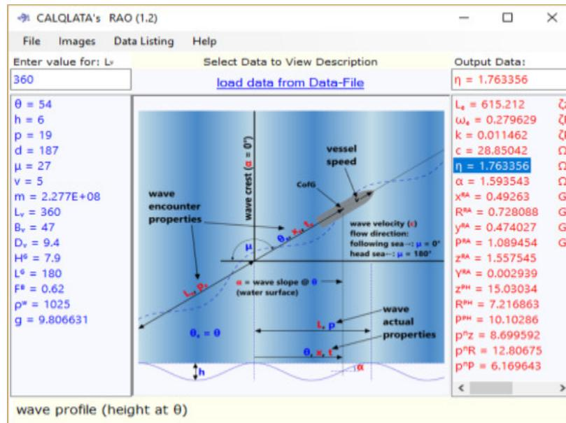
Fig. 4.19. Illustrative example of a RAO set of calculation for a specific vessel and metocean data input.
