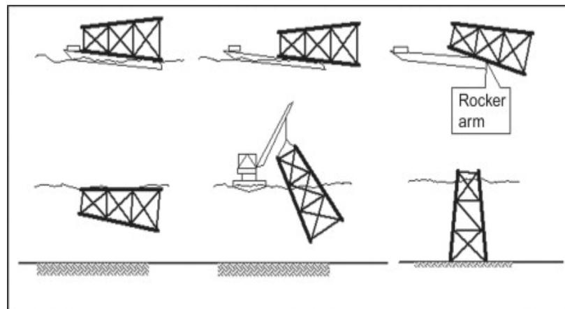
Figure 5.44. Launching and installing a jacket.
