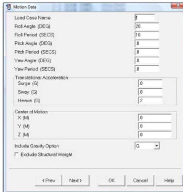
Figure 8.96. Motion input data in load case 1.
