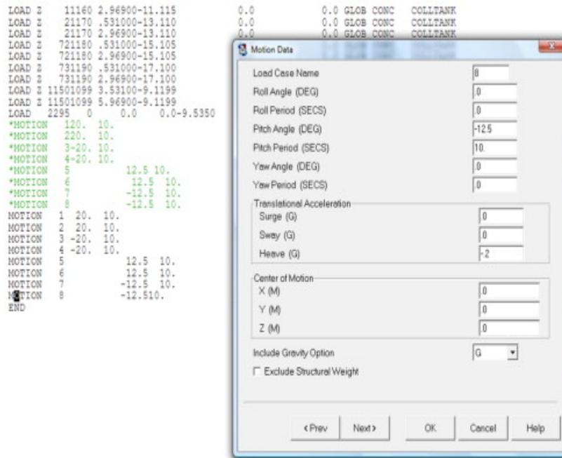
Figure 8.103. Motion input data in load case 8.
