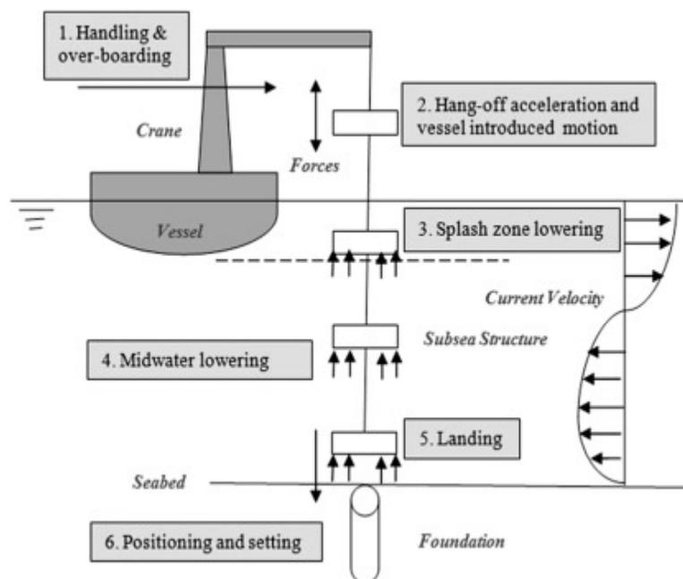
Figure 5-13. Sketch of Analysis Steps for Typical Subsea Structure.
