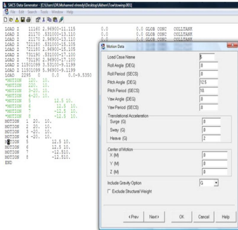
Figure 8.100. Motion input data in load case 5.
