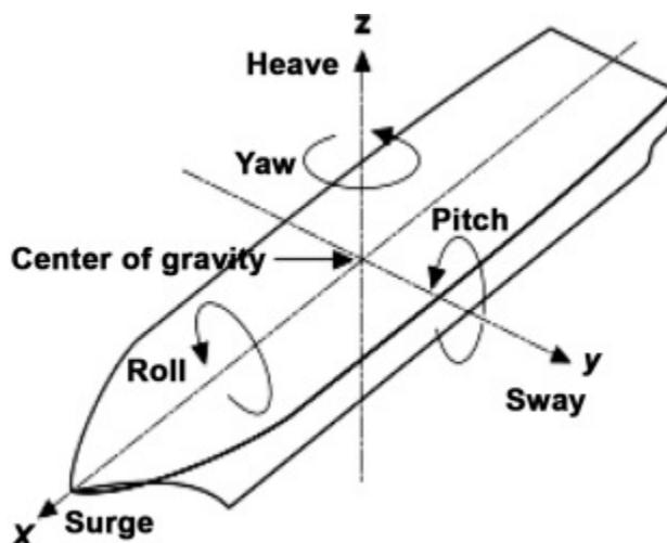
Fig. 4.18. Vessel's six degrees of freedom.
