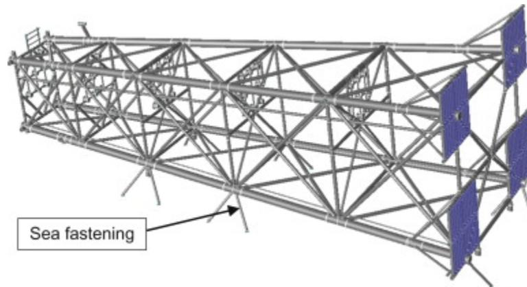
Figure 8.91. Sea fastening structure model.
