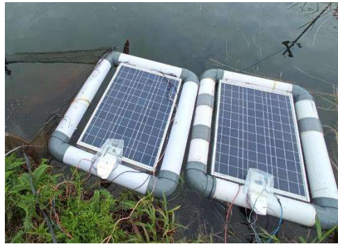
Figure 4. Floating photovoltaic panels
