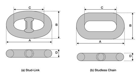
Figure 28. (a) Stud-link chain and (b) Studless chain.
