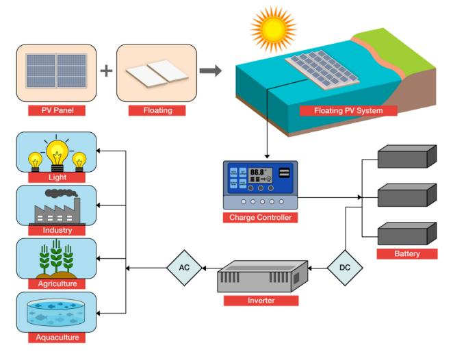
Figure 1. Diagram of a typical FPV system described in this review.
