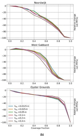
**Figure 15.** (a) Oyster Grounds (OG), West Gabbard (WG), and Noordwijk-10 (NW) sampling stations. (b) Relative change against the reference of net primary production with coverage for the three locations of the experiment and different values of roughness height of the platforms.
