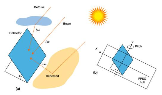
**Figure 13.** Solar radiation strikes a collector at a tilt angle (**a**). Location and orientation of the PV panel, effects of pitch motion; top view for case study 1 (**b**). Location and orientation of the PV panel, effects of roll motion; top view for case study 2.
