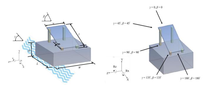
Figure 16. A schematic drawing of a tilting panel on a pontoon.
