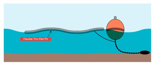
Figure 5. Schematic of the flexible floating PV concept.
