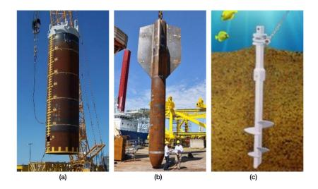
**Figure 34.** Pile anchor, torpedo anchor, and screw or helicoidal anchor respectively [101]. (**a**) Pile anchor, (**b**) torpedo anchor, and (**c**) screw or helicoidal anchor respectively.
