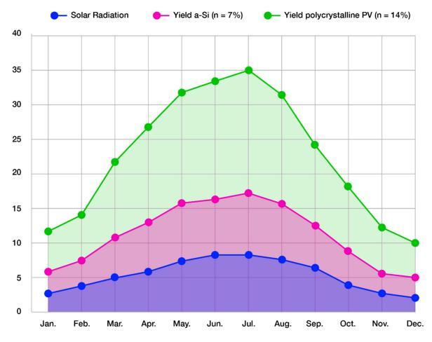
Figure 7. Malta solar and technical PV (horizontally oriented panels) resource averages.
