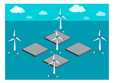
Figure 18. Combined floating wind and solar energy farm: general view.
