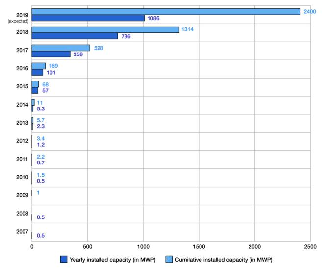
Figure 4. Global installations of floating solar PV.
