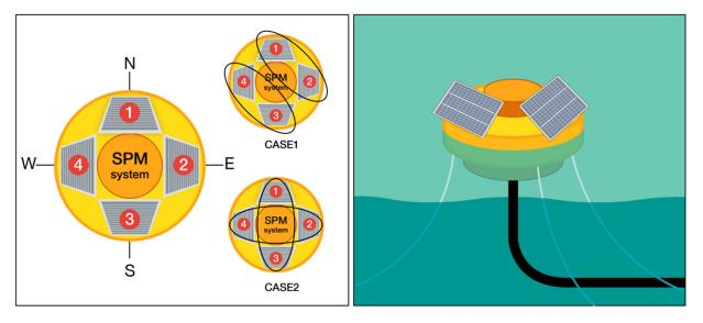
Figure 8. SPM (single point mooring) model with 4 panels (left) and SPM system (right).
