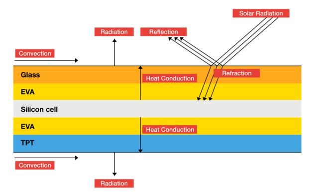
Figure 9. Sketch of the internal structure and heat transfer form of PV cells.
