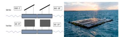
Schematic illustration of load cases on a 2 × 2 floating island. An offshore floating solar farm in the Dutch northern sea - Oceans of Energy technology
