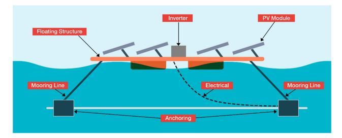
Figure 2. The main components of an FPV system.
