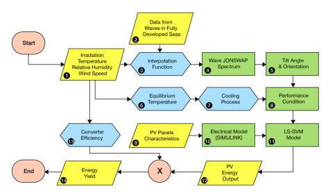
**Figure 12.** Model flowchart. JONSWAP (Joint North Sea Wave Project); LS-SVM (Least Square Support Vector Machine); PV (PhotoVoltaic).
