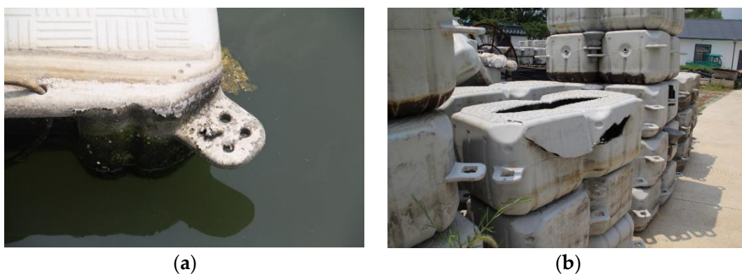
Figure 2. (a) Chalking of surface of float; (b) fracturing of outer layer of float.
