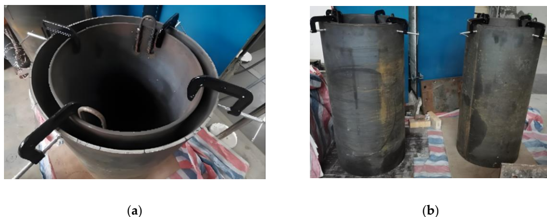
Figure 2. GJC specimens with mimicked defects: (a) the two steel tubes being assembled before pouring the grouting; (b) the GJCs specimens after pouring the grouting.
