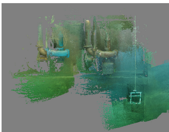
Fig. 7 Point cloud of the water filter (left) close up (right).
