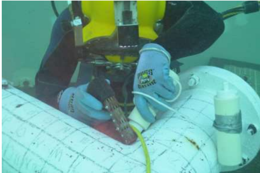
Figure 3. Magnetic Particle Methods testing underwater (CoreIRM, 2019)
