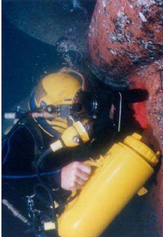
Figure 3. Eddy Current Methods testing underwater
