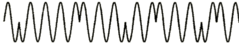
Section of biphasic modulated spread spectrum ultrasonic waveform
