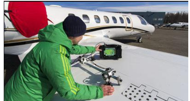
Place the probe at the surface of specimen
