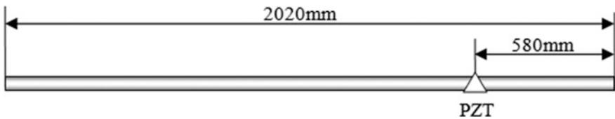
**Fig. 3** The installation location of the PZT in the rope
