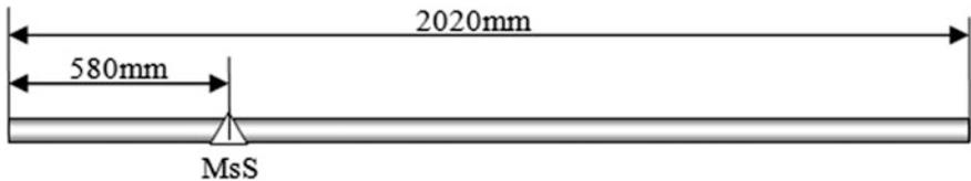
Fig. 5 The installation location of the MsS in the rope
