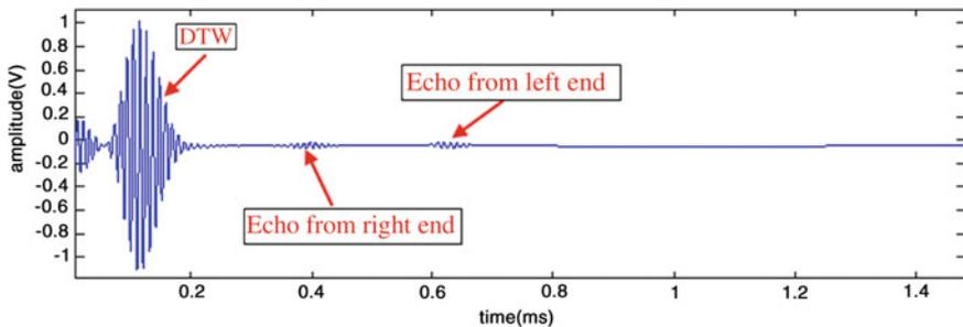
**Fig. 8** The reflected signal waveform received by MsS when the PZT was working as the transmitter
