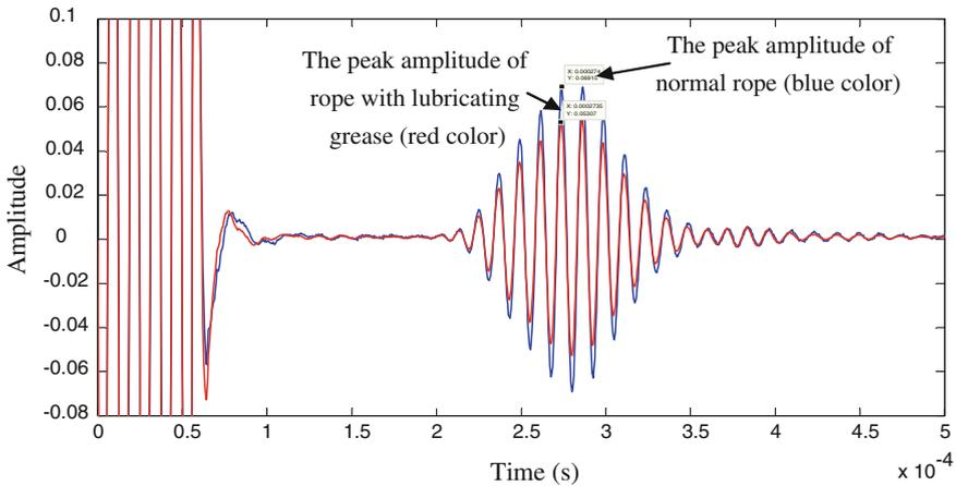
**Fig. 16** The comparison on the received signal waveform from rope with/without lubricating grease
