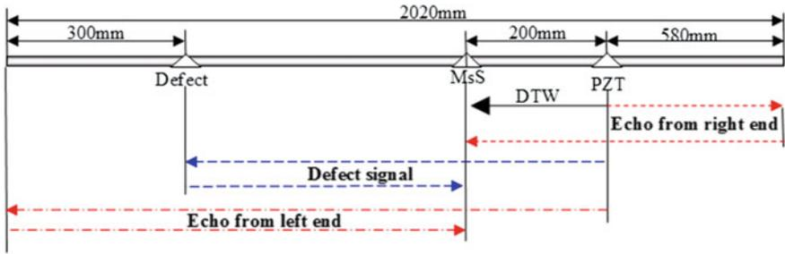
Fig. 10 Locations of PZTW and MsS onto the wire rope and propagation paths of guided wave
