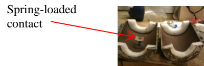
Figure 18: Pinhole leak with spring loaded contact
