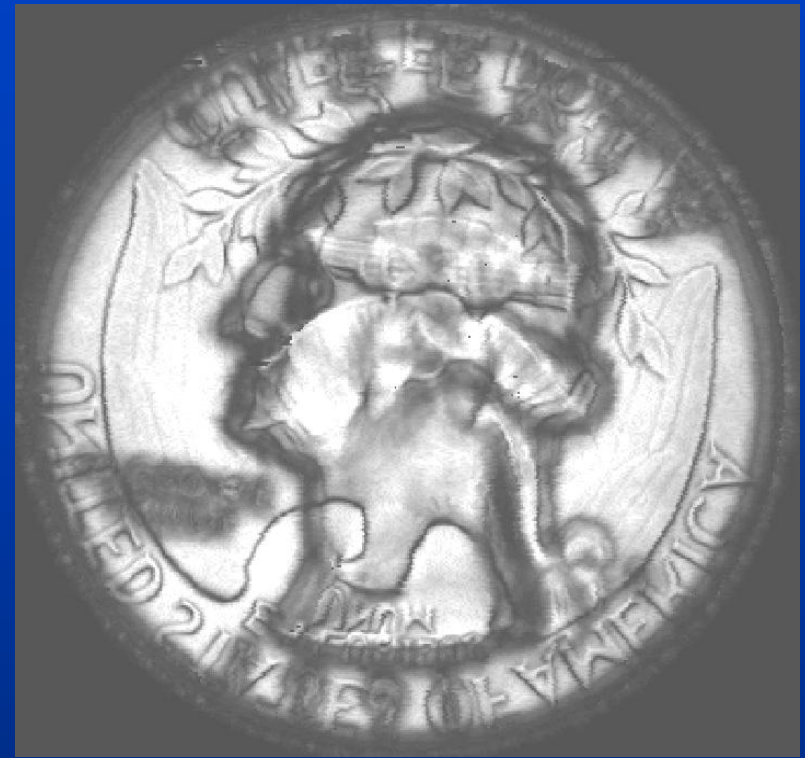
Gray scale image produced using the sound reflected from the back surface of the coin (inspected from "heads" side)
