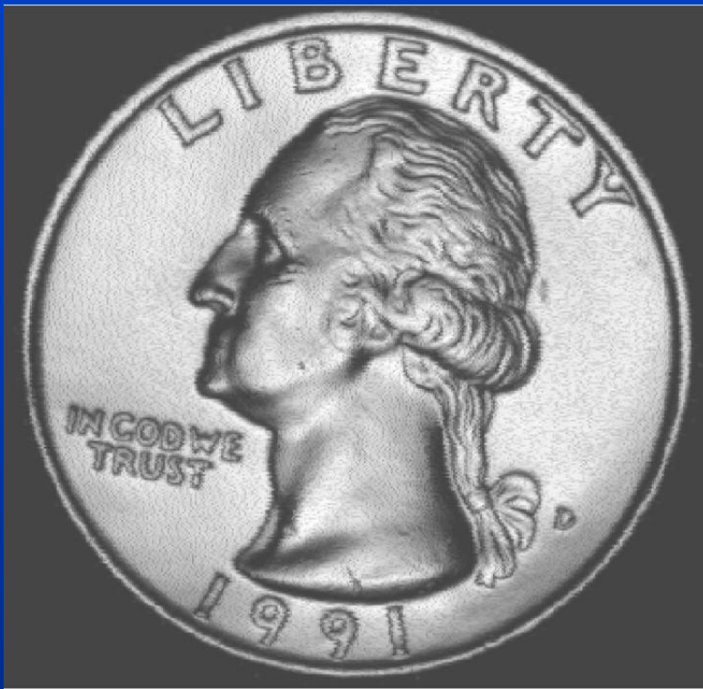
Gray scale image produced using the sound reflected from the front surface of the coin
