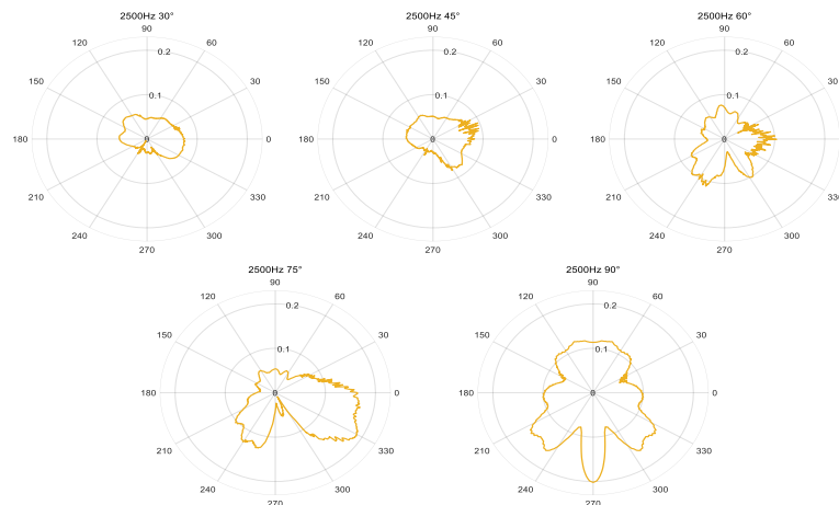
Figure 9. Scattering pressure characteristics of the buried pipeline 1 meter from the center of the pipeline
