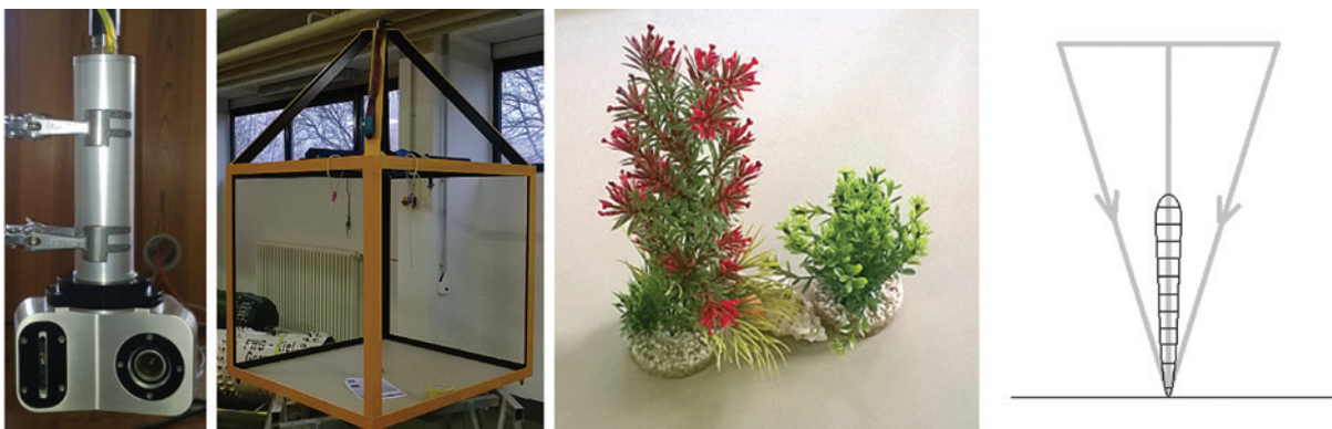
Figure 2: From left to right: ULS-100 system owned by WTD 71, frame with an edge length of 1 m, artificial plants enclosing a shell on the sand-colored bottom plate of the frame, and principle of LOS. The ULS on the left consists of the lower part of the sensor head and of the upper part of a cylinder containing a stepping motor for rotating the sensor head. The sensor head is equipped with the laser line scanner on the left and the camera optics on the right-hand side.
