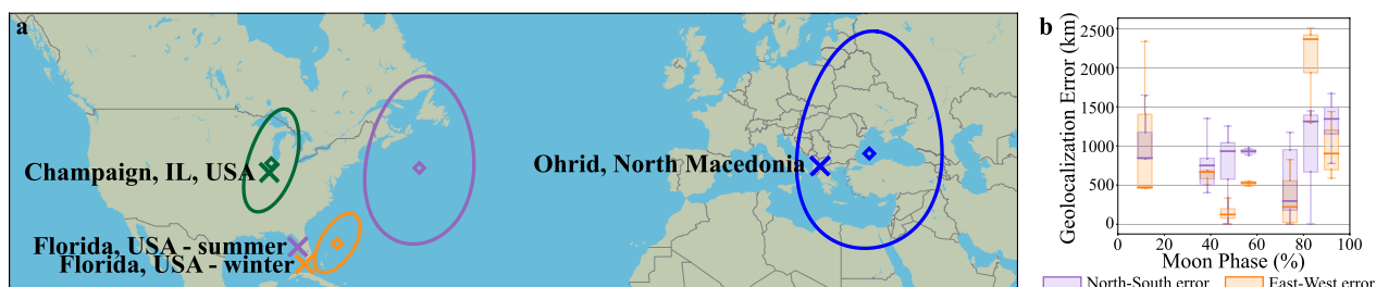
Fig. 9 Geolocalization accuracy during nighttime under different moon phases. a The global map displays the mean (represented by a diamond) and first standard deviation (represented by a solid line) of the particle filter estimate of geolocation at the four sites (crosses) during the new moon and full moon phases. b The box plots indicate the median and upper/lower quartiles for the North–South (purple) and East–West (orange) geolocalization prediction errors
