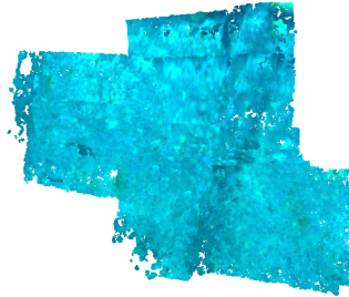
Fig. 7: Shipwreck's partial point cloud from the stereo dense 3D mapping pipeline.
