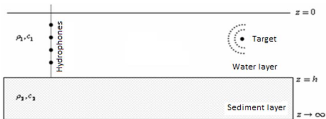
A schematic view of the Pekeris waveguide.
