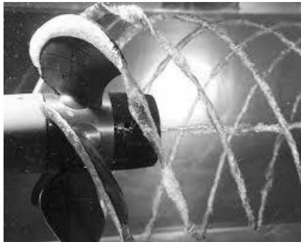
The hydrodynamic propeller cavitation.
