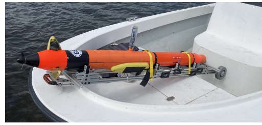
Fig. 6. Riptide Micro-UUV with modified payload
