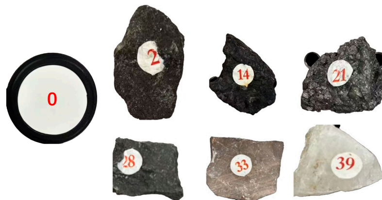
Figure 3. Selected seven targets with different reflectivity: Num.0: reflective plate (0.97); Num.2: manganese ore (0.23); Num.14: coal (0.25); Num.21: graphite (0.35); Num.28: basalt (0.29); Num.33: limestone (0.48); Num.39: quartzite (0.53).
