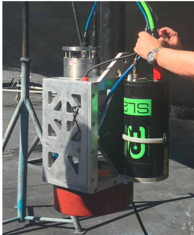
Figure 2. View of the mounting system showing the 3DAD SL2 unit, the ROVINS, and the sonar transducer.
