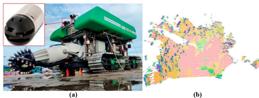
Figure 11. The tracked underwater robot with FLS and the mapping result of the sea trial. (a) the tracked deep-sea underwater robot (b) the mapping result of the sea trial.
