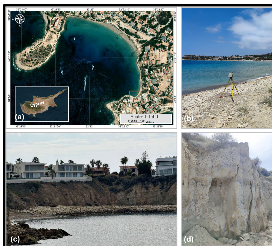
Figure 3. (a) The study area with TLS (red box), (b) TLS—Leica Scanstation C10, (c) frontal view of the sea cliff at Coral Beach, (d) detachment surfaces and debris cones at the cliff toe.
