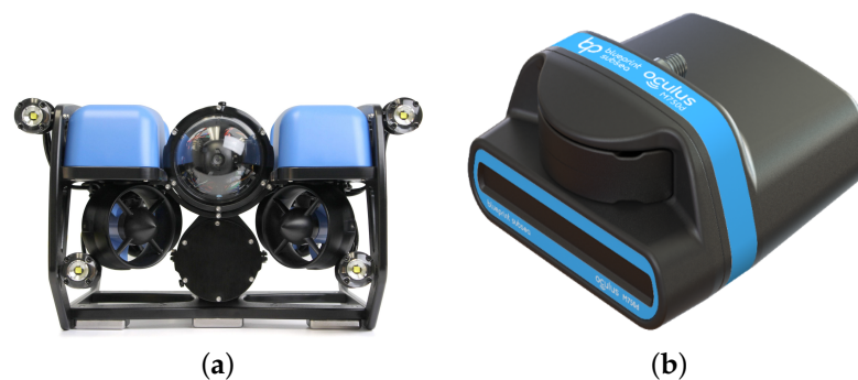
Figure 1. Underwater vehicles and sonar. (a) BlueROV, (b) m750d sonar. The BlueROV has the capability of submerging to a depth of 100 m and can be equipped with multiple attachments, such as clamps or scanning sonar. The Oculus m750D multi-beam imaging sonar features two working frequencies: 750 kHz/1.2 MHz, with the detection range of 120 m/40 m, respectively.
