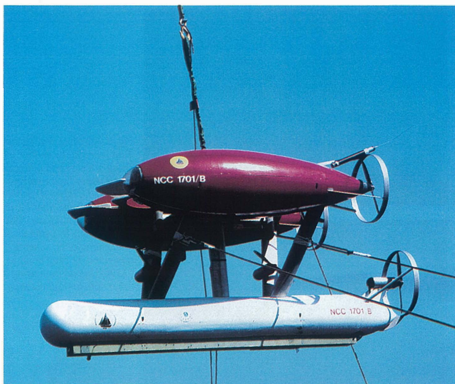
Fig. 1. Photo showing the autonomous underwater vehicle ABE being launched. The upper red pods contain flotation, acoustic navigation transponders, and video cameras. The pressure housing (white, lower center) contains the main electronics, batteries, and magnetic sensor.
