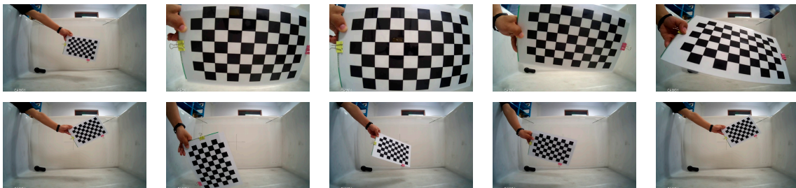
Figure 4. Images captured in the air (without water, used for obtaining initial parameters).
