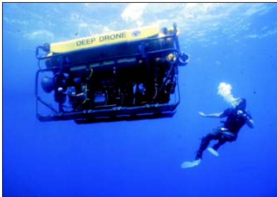
Figure 13-2. Remotely Operated Vehicle (ROV) Deep Drone.
