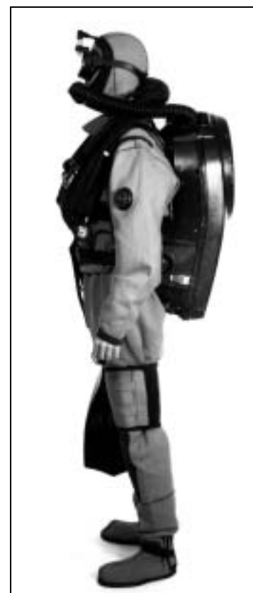
Figure 17-1. MK 16 MOD 0 Closed-Circuit Mixed-Gas UBA.
