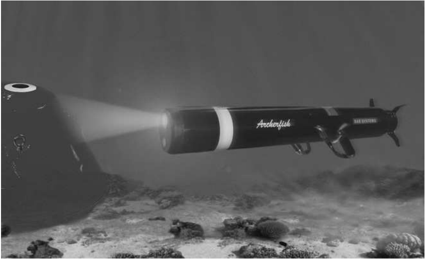
Figure 9.6 Archerfish prosecuting bottom mine (courtesy BAE Systems).
