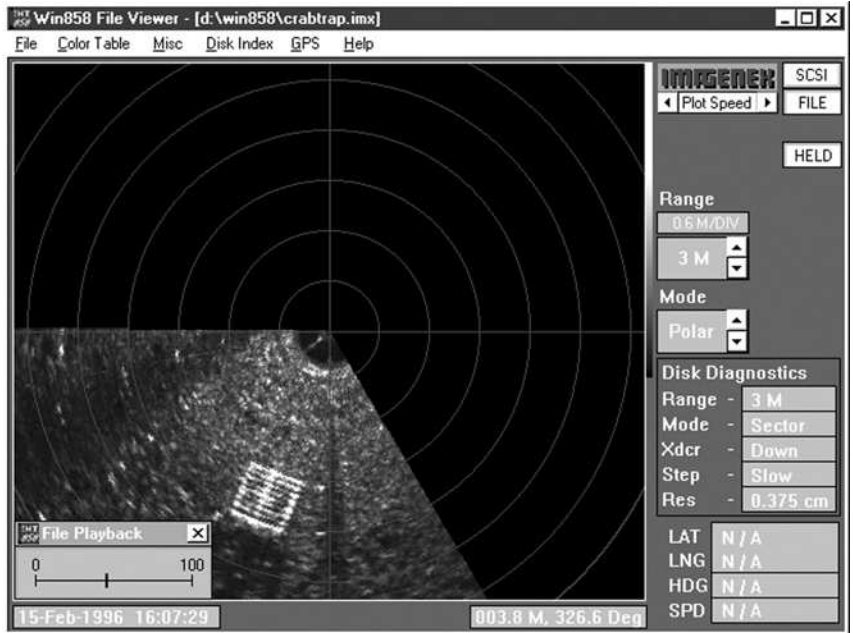
Figure 5.29 Sonar scan of a crab trap with imaging sonar.
