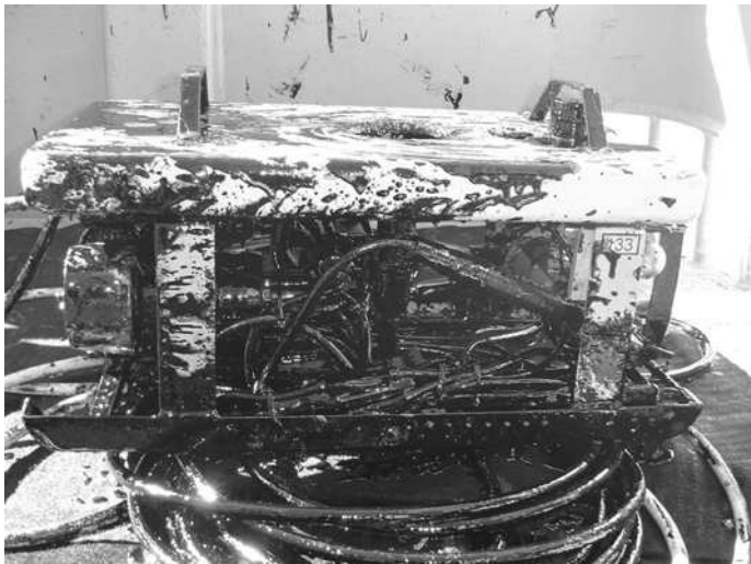
Figure 12.9 ROV contaminated during an oil spill survey.
