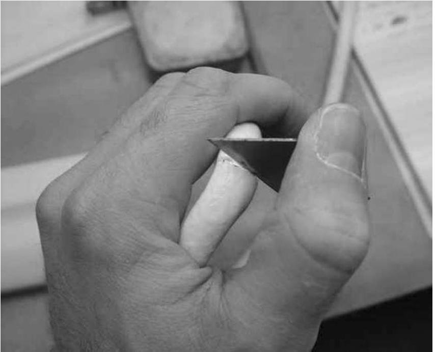
Figure 3.18 Slicing is conducted by peeling back the conductors of the tether.
