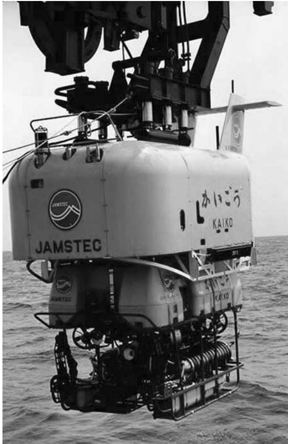
Figure 1.7 Kaiko – the world's deepest diving ROV.
