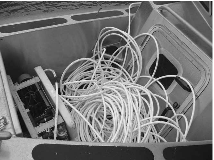
Figure 8.8 Large ROV aboard response boat showing excess green tether.
