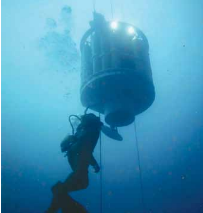
Lock-out diving bells, developed from the 1960s onwards, freed divers from the tyranny of time and enabled them to work more productively and effectively on deep water projects.
