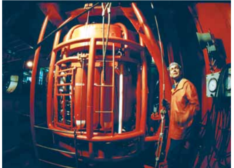
Lock-out diving bells, developed from the 1960s onwards, freed divers from the tyranny of time and enabled them to work more productively and effectively on deep water projects.
