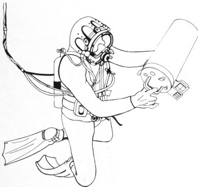
Figure 6-28 Revised lightweight diving outfit includes the diver's mask USN MK 1 and wet suit.
