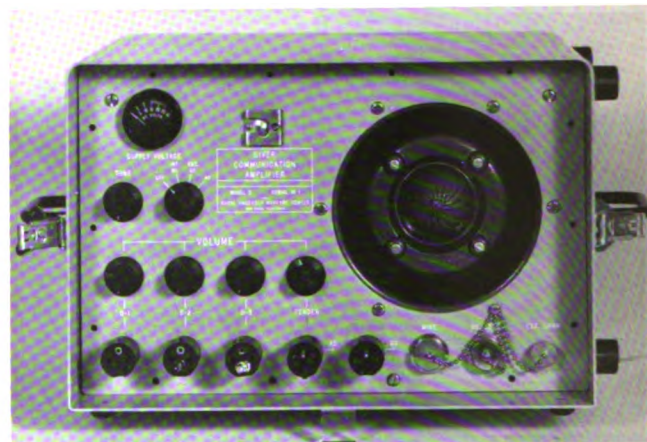
Figure 6-58 Model 2 Diver's Intercommunication System.
