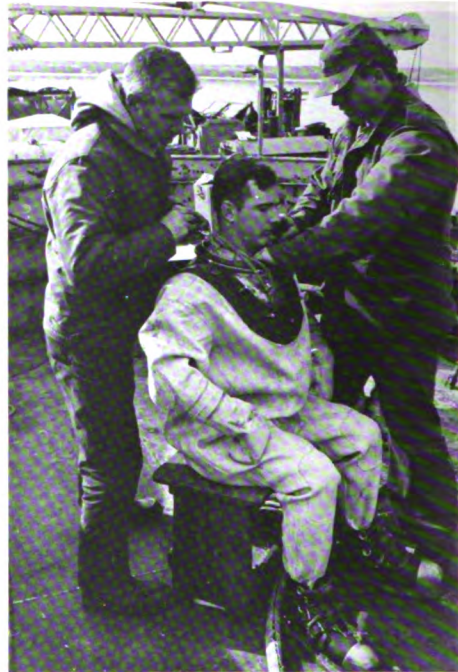
H With the diver seated, the breastplate is positioned. Note that the breastplate fits between the canvas suit and the rubber gasket.
