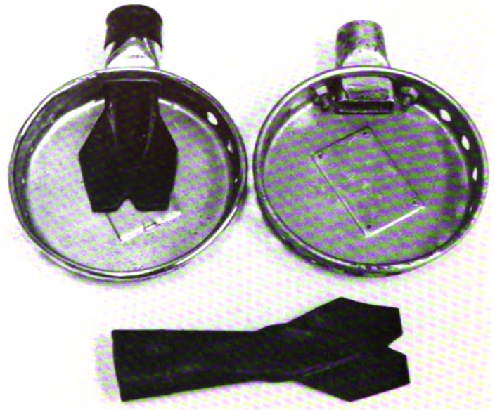
Figure 5-8 Flutter valve in double hose demand regulator
