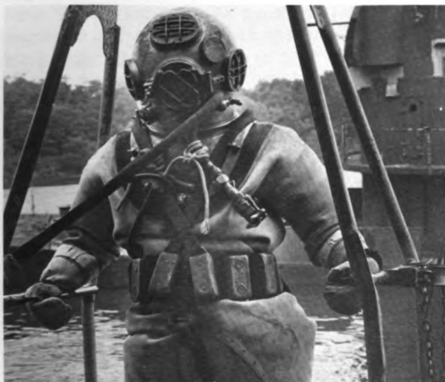
Figure 6-15 Communication/life-line, air hose, and pneumofathometer in use for deep-sea diving.
