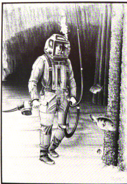
Figure 6-36 Mark 12 Surface-Supported Diving System (SSDS).
