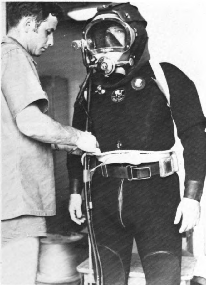
M A lifeline is secured around the diver's waist.
