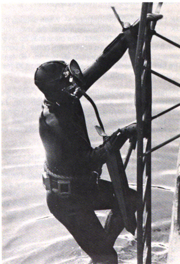
Figure 6-19 Lightweight diving gear shown with Jack Browne mask and wet suit.
