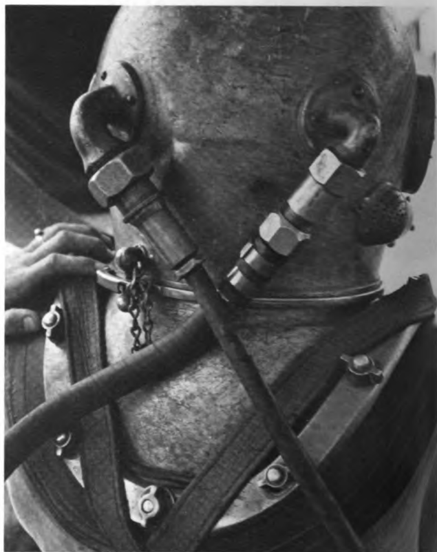
Figure 6-13 Air hose, communications cable and fittings shown properly secured to diver.
