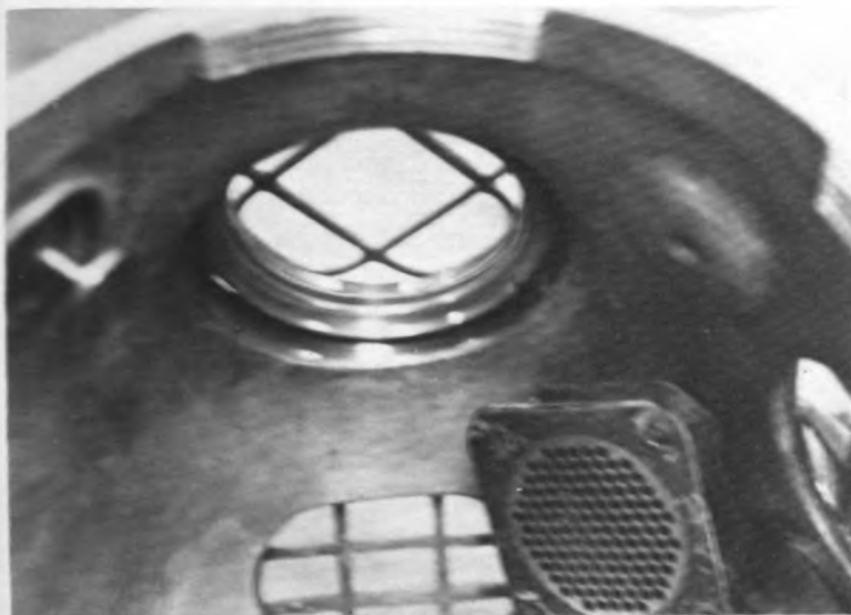
Figure 6-5 Interior view of helmet. Note location of reproducer and chin button.
