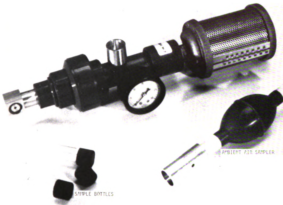
Figure 6 Ambient Air Sampler and Sample Bottles shown with High Pressure Sampler
