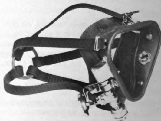
Figure 6-33 Standard lightweight masks, with control valve attached through an inhalation valve (upper); and control valve attached directly through an elbow (lower).
