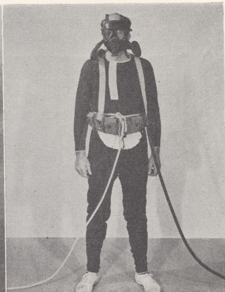
Converted MK III gas mask diving rig.
