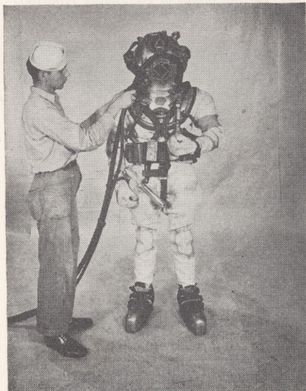
Front view of diver in complete outfit of the helium-oxygen deep sea diving outfit.
