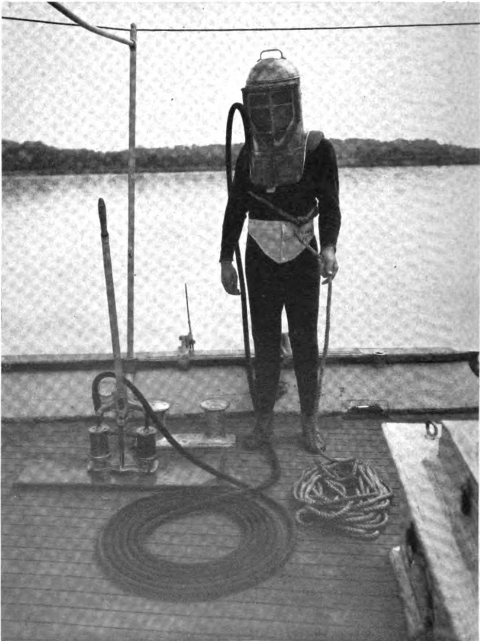
PLATE 76.—Shallow water diving apparatus—Miller-Dunn type.
