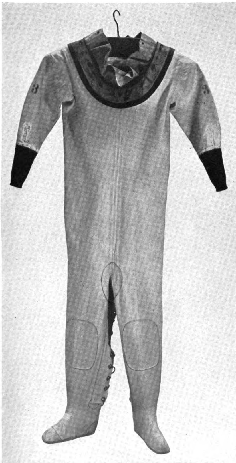
PLATE 20.—Standard diving dress, with cuffs attached—Front view.
