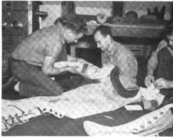
PLATE 5—FIGURE 2.—Diving suit repair work.
