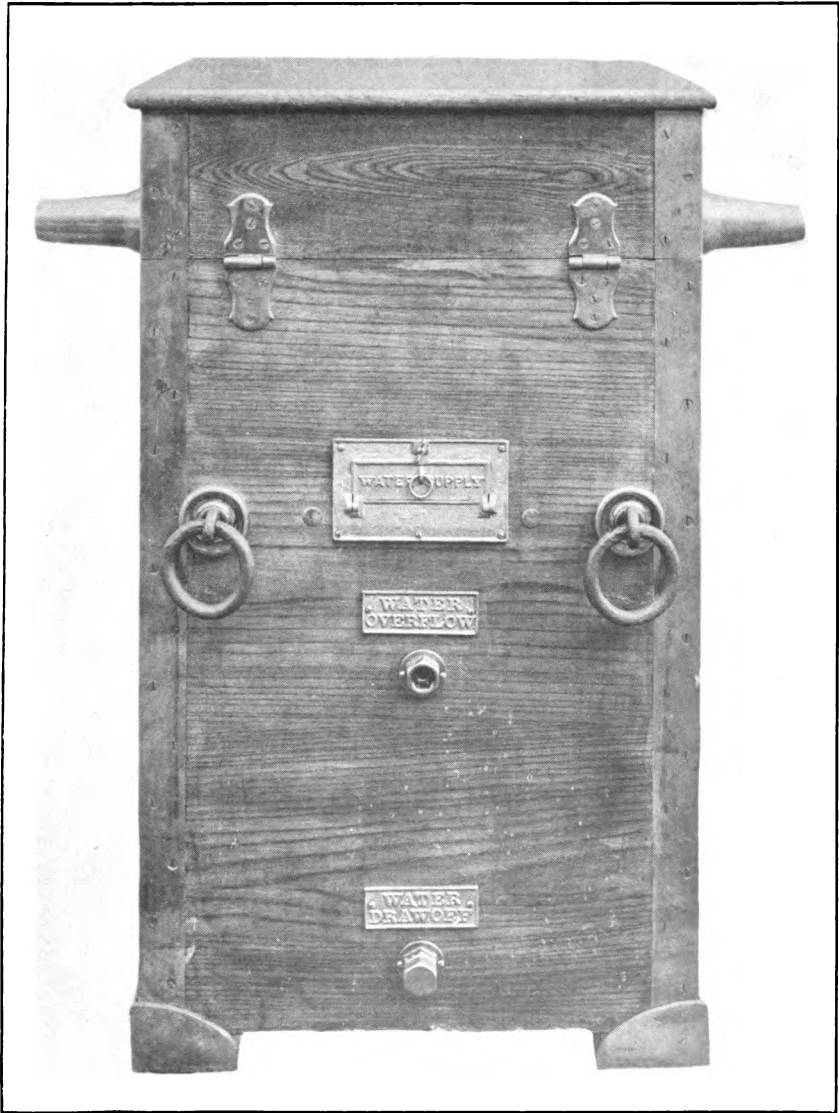
DIVING AIR PUMP MARK III, BACK VIEW.
