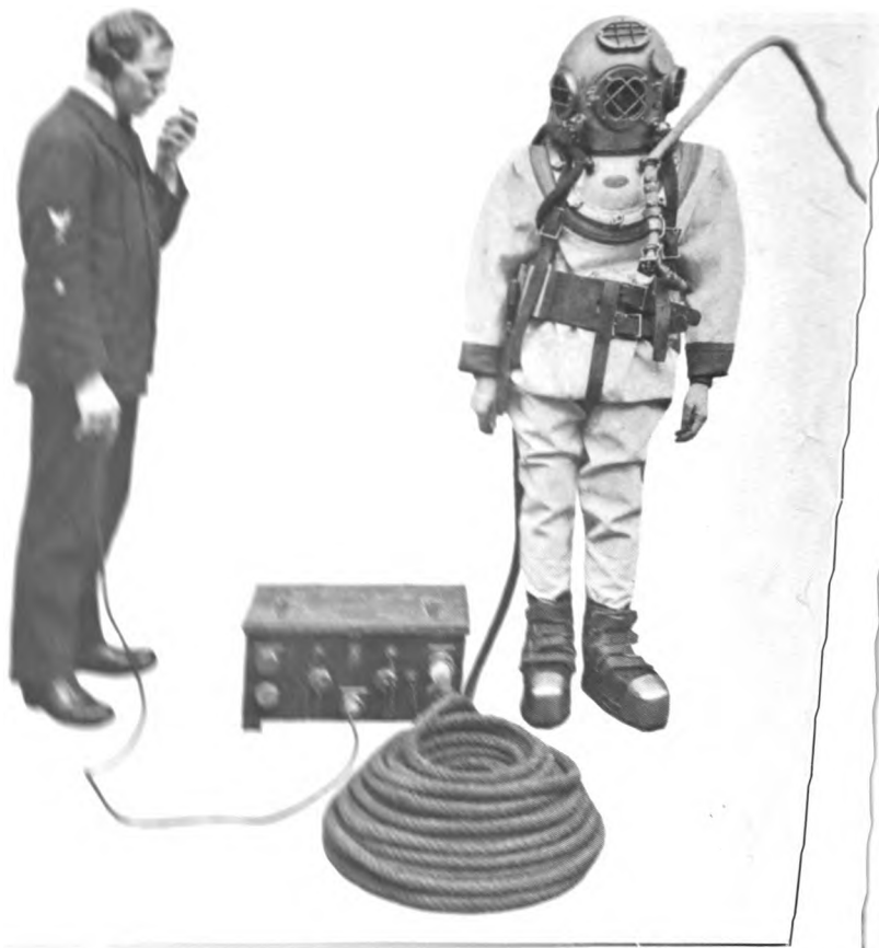
A DIVER'S SUIT AND ACCESSORIES WITH TELEPHONE.
