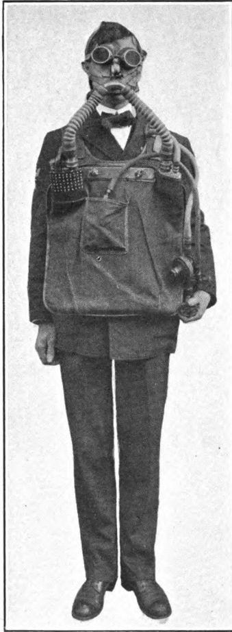
OXYGEN RESCUE APPARATUS. PROTOTYPE, FRONT VIEW.
