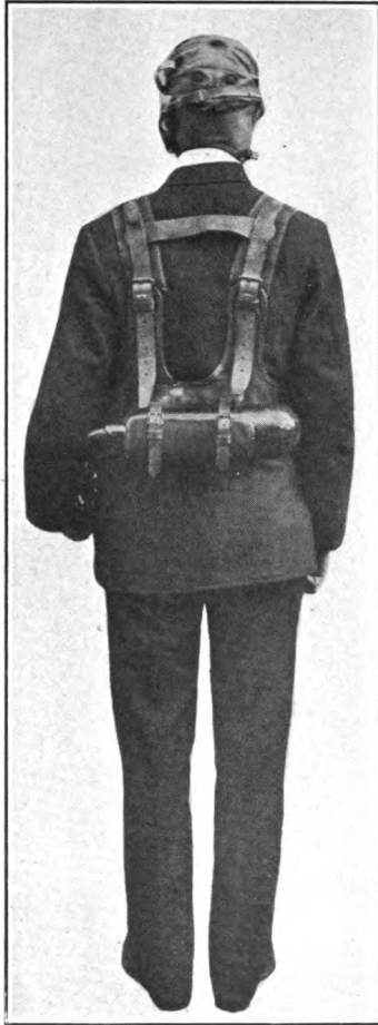
OXYGEN RESCUE APPARATUS. PROTOTYPE, BACK VIEW.
