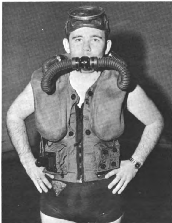
FIGURE D-21.—Oxygen recirculating underwater breathing apparatus—front view.
