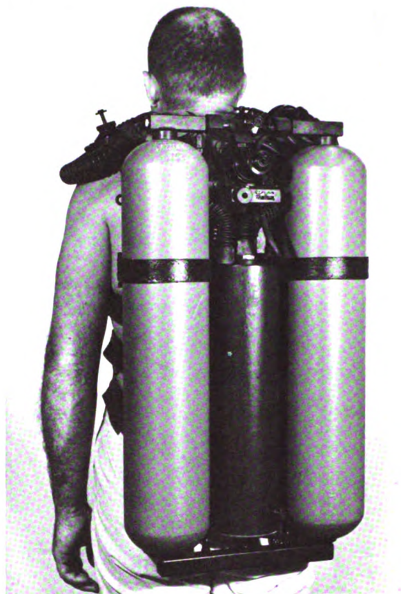
FIGURE 3-35.—Pure-oxygen recirculating, underwater breathing apparatus (back view).
