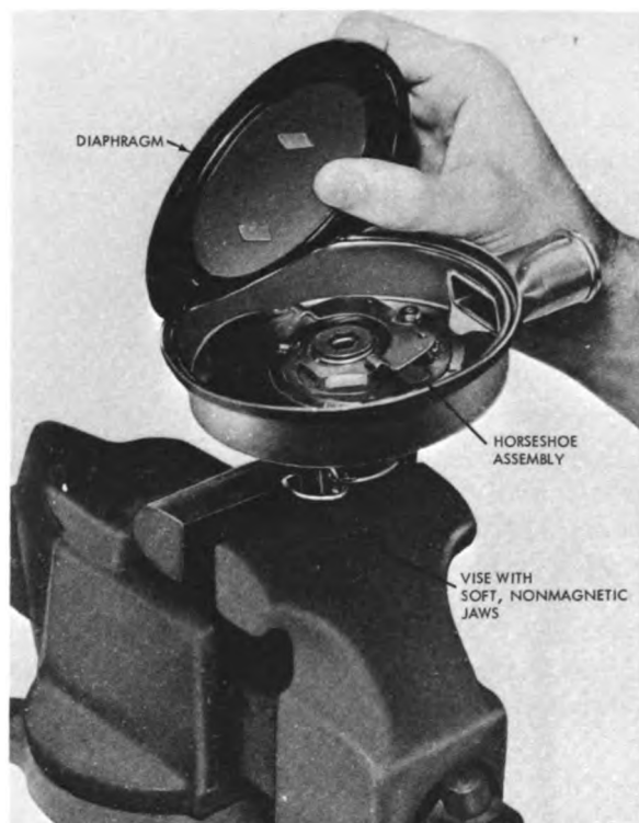
FIGURE D-14.—Locating low-pressure diaphragm with respect to horseshoe extremities.
