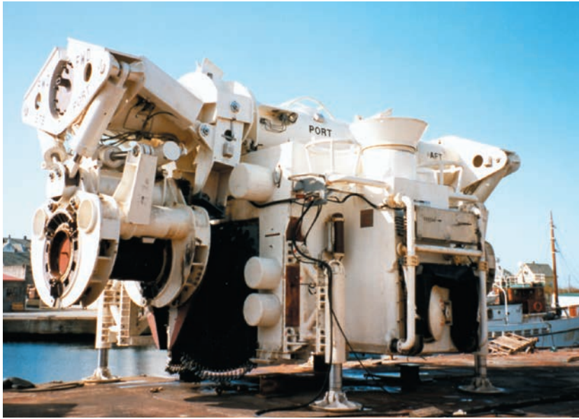
A welding habitat on land. The structures required to weld in dry conditions under water were large and complex.
