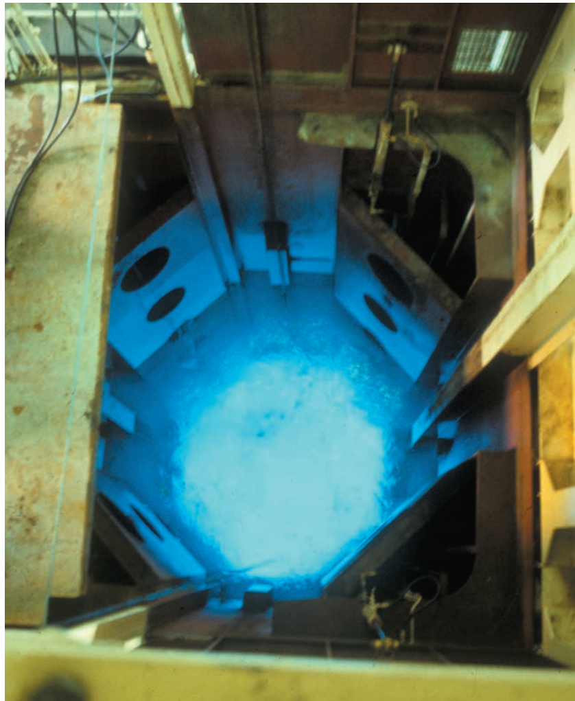
The moonpool, a shaft through the bottom of the ship where the diving bell was lowered into the sea.
