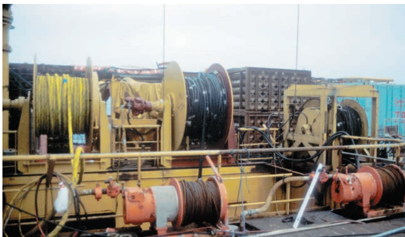
Extensive diving called for large quantities of equipment – breathing gas and drums holding umbilicals, hoses and wire cables. Photo: Bjørn Wilhelm Kahrs
