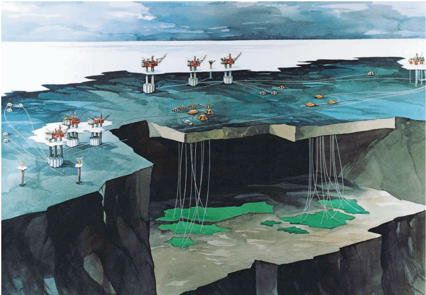
Statfjord satellites tied back to the main field. Photo: Statoil
