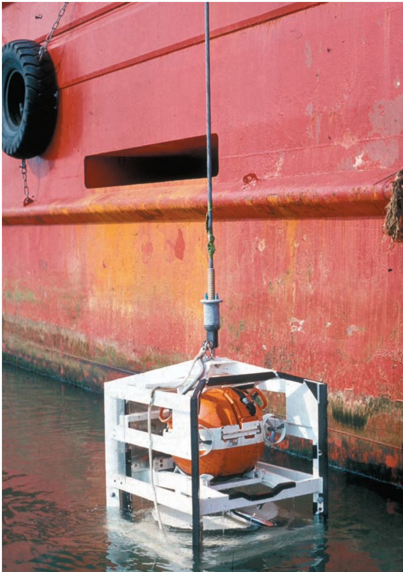
An RCV 225 eyeball was used on Ekofisk for visual inspection of drilling operations and monitoring divers to enhance their safety. Photo: Tor Jan Wiik
