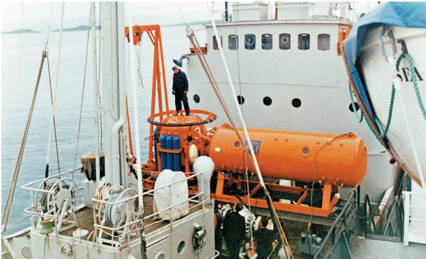
The Rat Trap (left, with man standing on top) ready to blast free a subsea wellhead in 1972-73. Photo: Leif-Tore Skjerven
