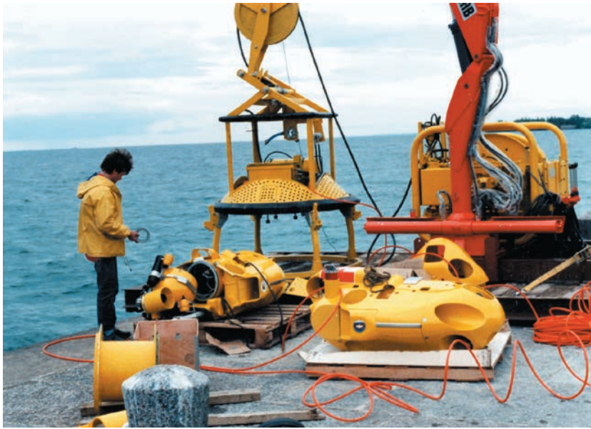
An inspection ROV is serviced before being placed in its “garage” and submerged in the sea, ready for new assignments.
