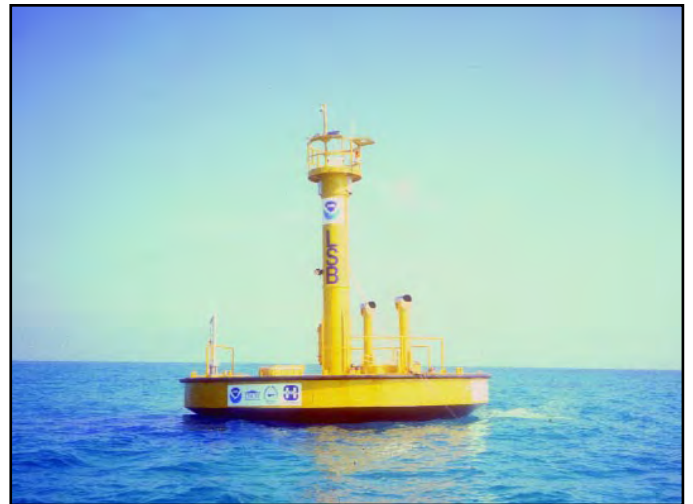
FIGURE 11.11 Life Support Buoy (LSB) for Aquarius 2000
