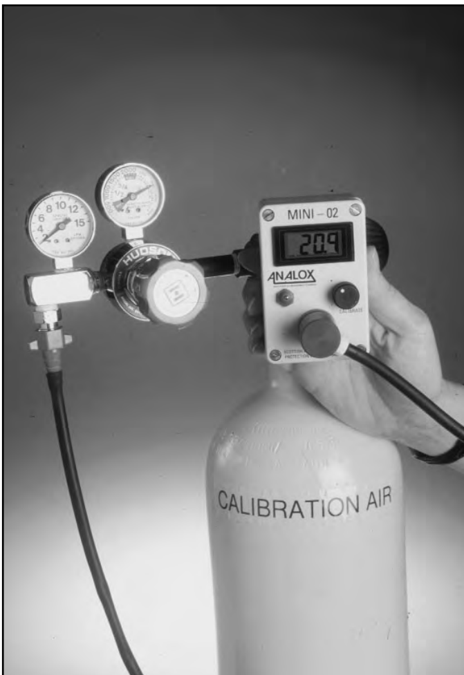
FIGURE 15.19 Oxygen Analyzer, with Flow Meter Set to 2 lpm
