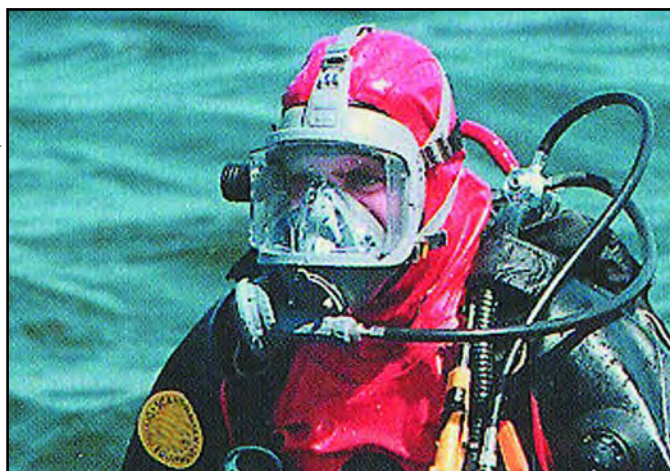
FIGURE 5.55 Full-Face Masks With Voice Communicators
