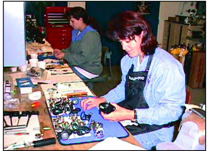
FIGURE 5.20 NOAA Technician Inspecting and Repairing Regulators
