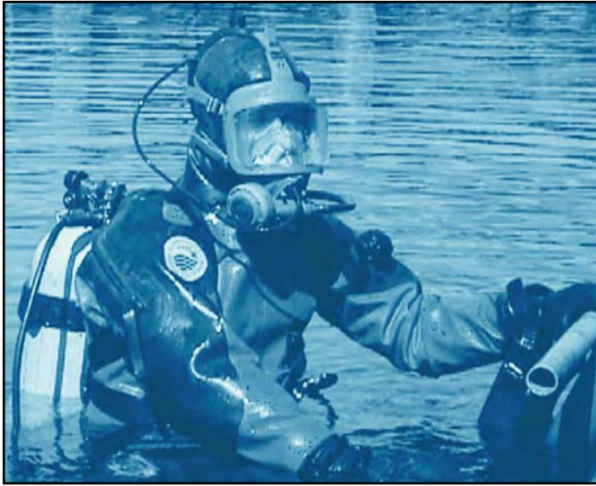
FIGURE 13.6 Full-Face Mask with Dry Suit
