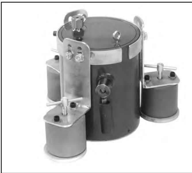
FIGURE 10.22 Explosive Hole Punch
