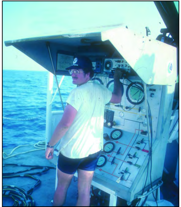
FIGURE 11.22 Diver/Open-Bottom Bell System Control Panel
