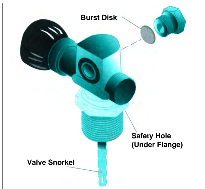
FIGURE 5.26 Cylinder Valve Safety Features
