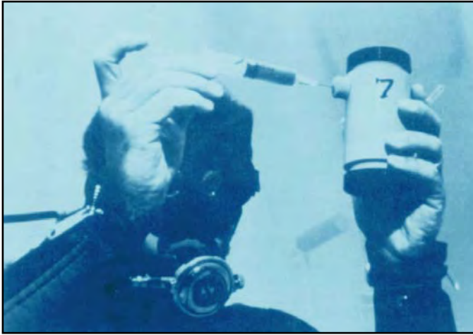
FIGURE 9.37 Custom Dissolved Oxygen Water Sampler
