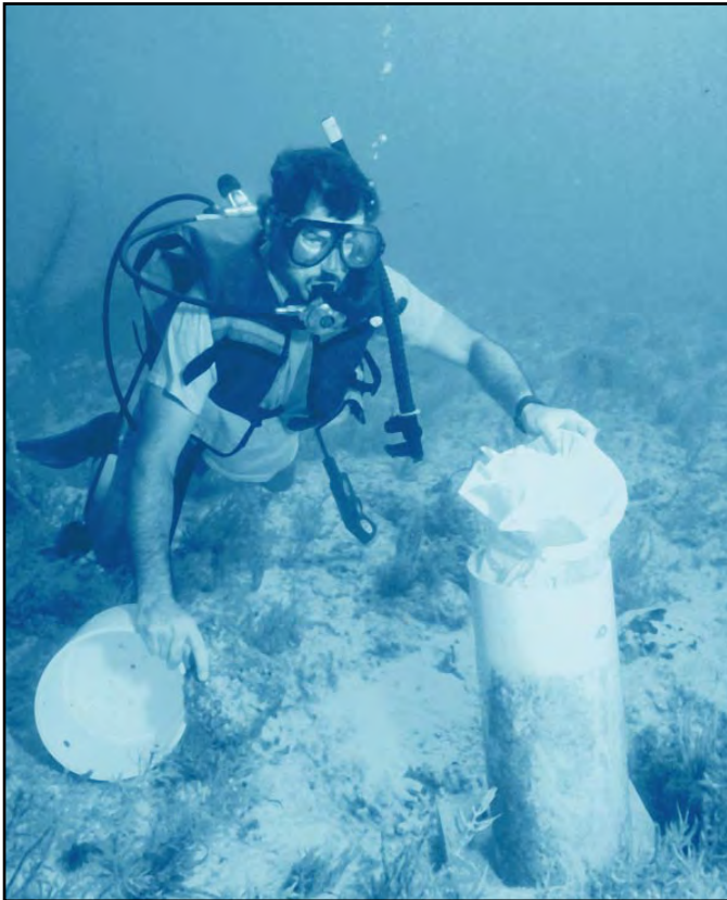
FIGURE 9.33 Deploying an Instrument Inside PVC Housing
