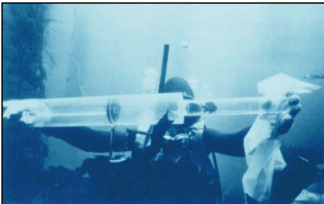
FIGURE 9.48 Slurp Gun Used to Collect Small Fish
