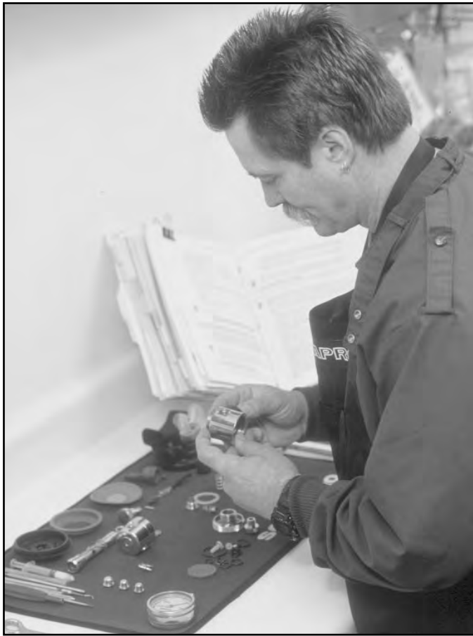
FIGURE 15.10 Preparation of Regulator Parts for Oxygen Service
