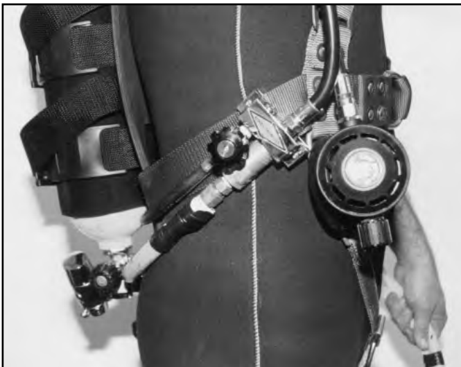
FIGURE 5.58 Emergency Air Cylinder Integrated With the Air Hose
