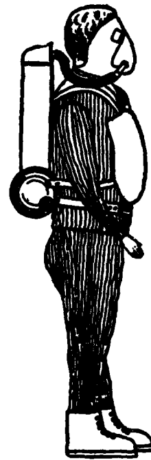
Figure 9-1 Fleuss Apparatus; the first oxygen recirculating breathing apparatus.
