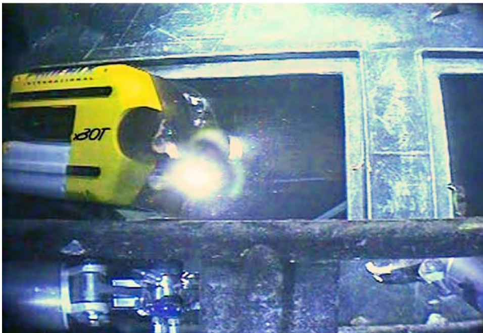
Figure 5-22. Phoenix's xBot entering the bridge control room window. Photo taken from Deep Drone.
