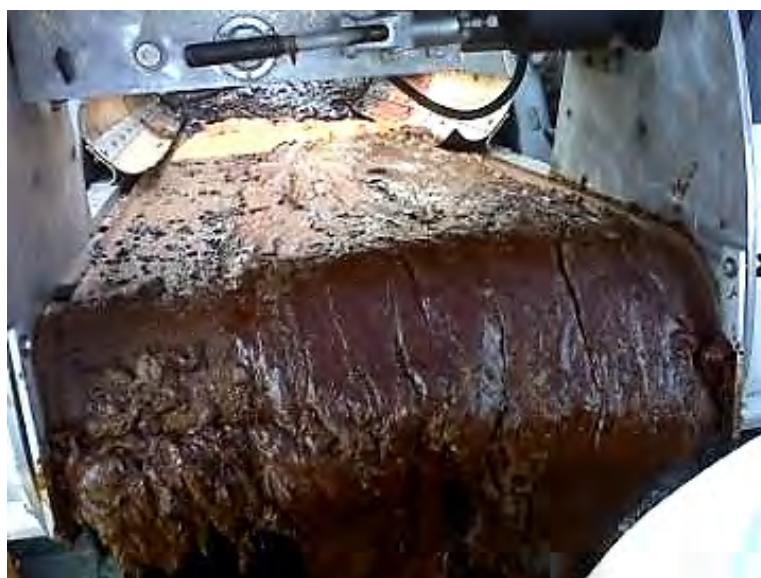
Figure 16. Crude Oil Rolling off Skimmer Belt
