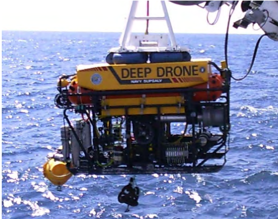
Figure 5-20. SUPSALV's Deep Drone deploying off M/V GENNIE LAB. In the portside manipulator is the transponder float and hanging under Deep Drone is the weight used to hold the transponder in position on the Gulf floor.
