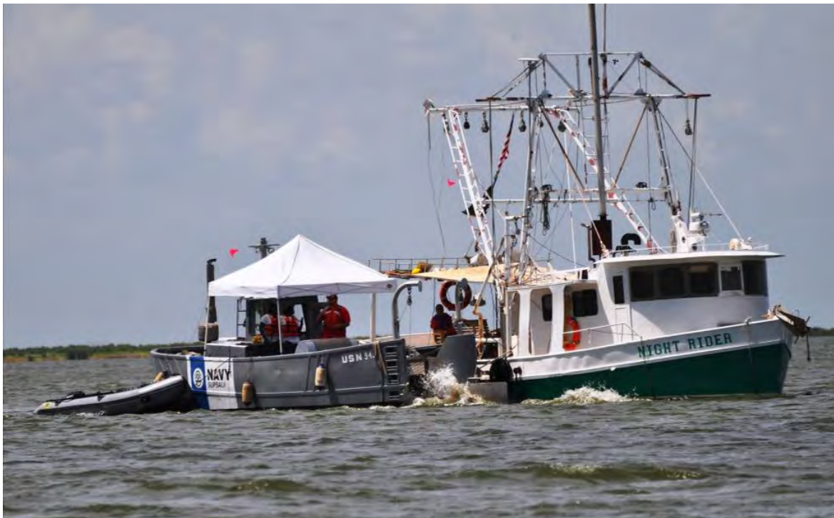
Figure B-7. Class V Vessel Skimmer in Hip-Tow Configuration with Grand Isle Based Shrimp Boat, Night Rider
