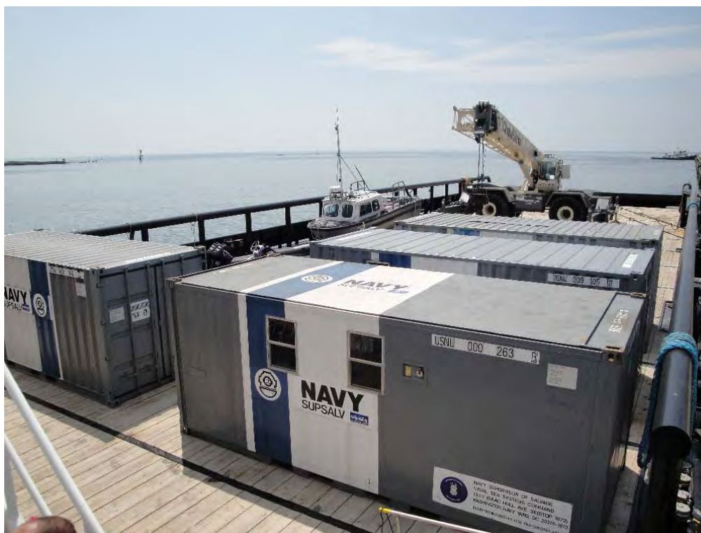
Figure 5-8. Stern deck of OSV BAYOU BEE configured with crane and shop vans to provide mobile MARCO Class V skimmer maintenance.
