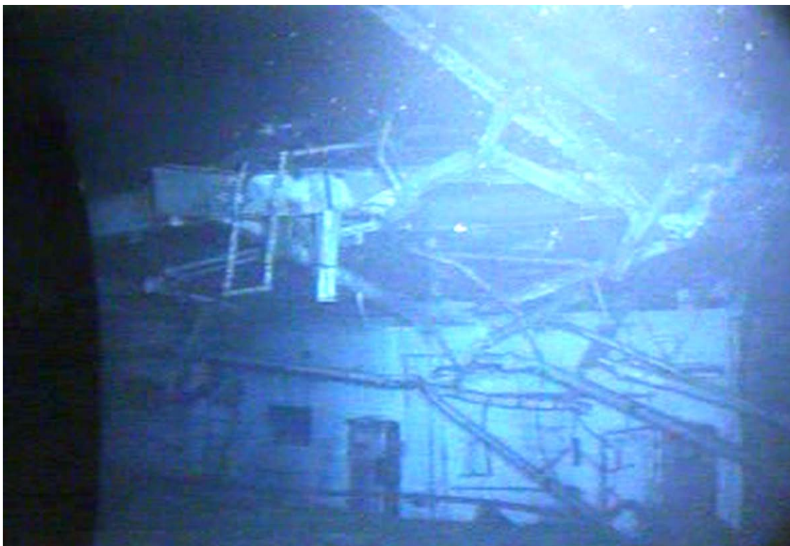
Photograph 14: Bridge Control Room with Helicopter Deck Wreckage
