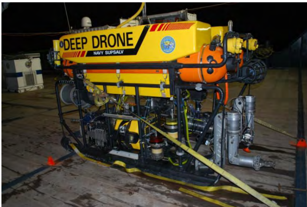
Photograph 8: Deep Drone with xBot Ready to Launch
