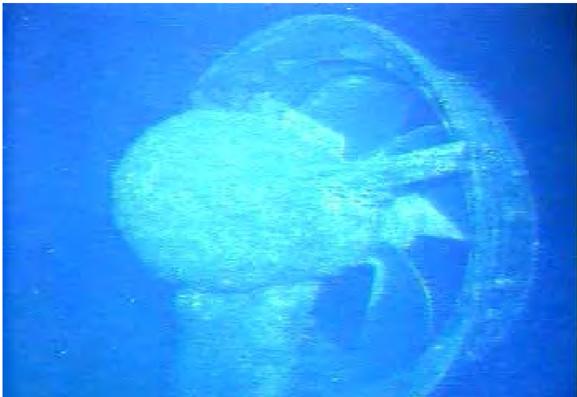
Photograph 9: Deep Water Horizon Megastar Thruster Pod
