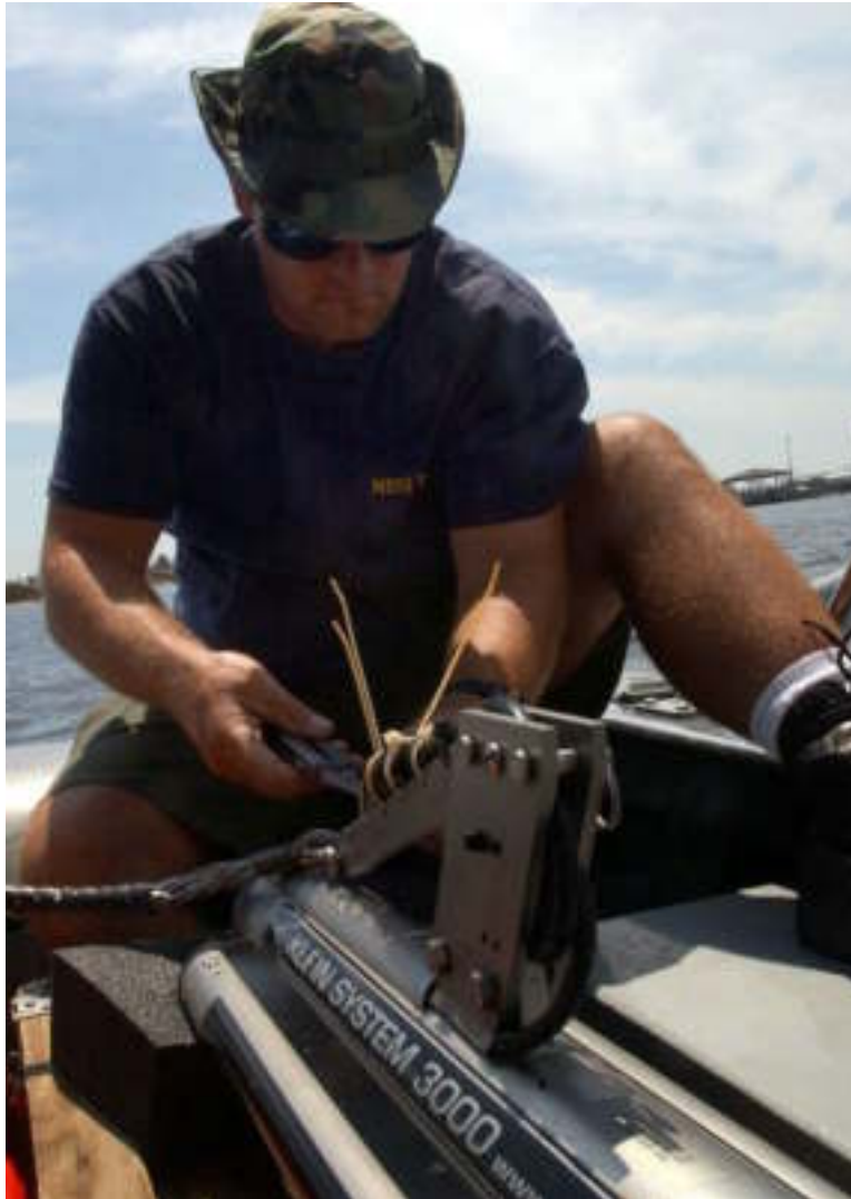
Figure 5-19. Damage Controlman 1st Class Christopher Daly, assigned to Mobile Diving and Salvage Unit Two, prepares a towed sonar to survey the channel leading into Naval Station Pascagoula, MS, to search for large debris hidden beneath the waters as part of the Hurricane Katrina aftermath repairs.
