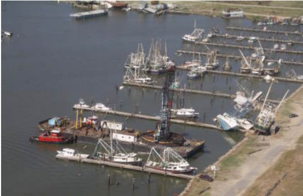
Figure 5-9. Donjon's Columbia New York lifting fishing boats in the marina in Venice, LA.
