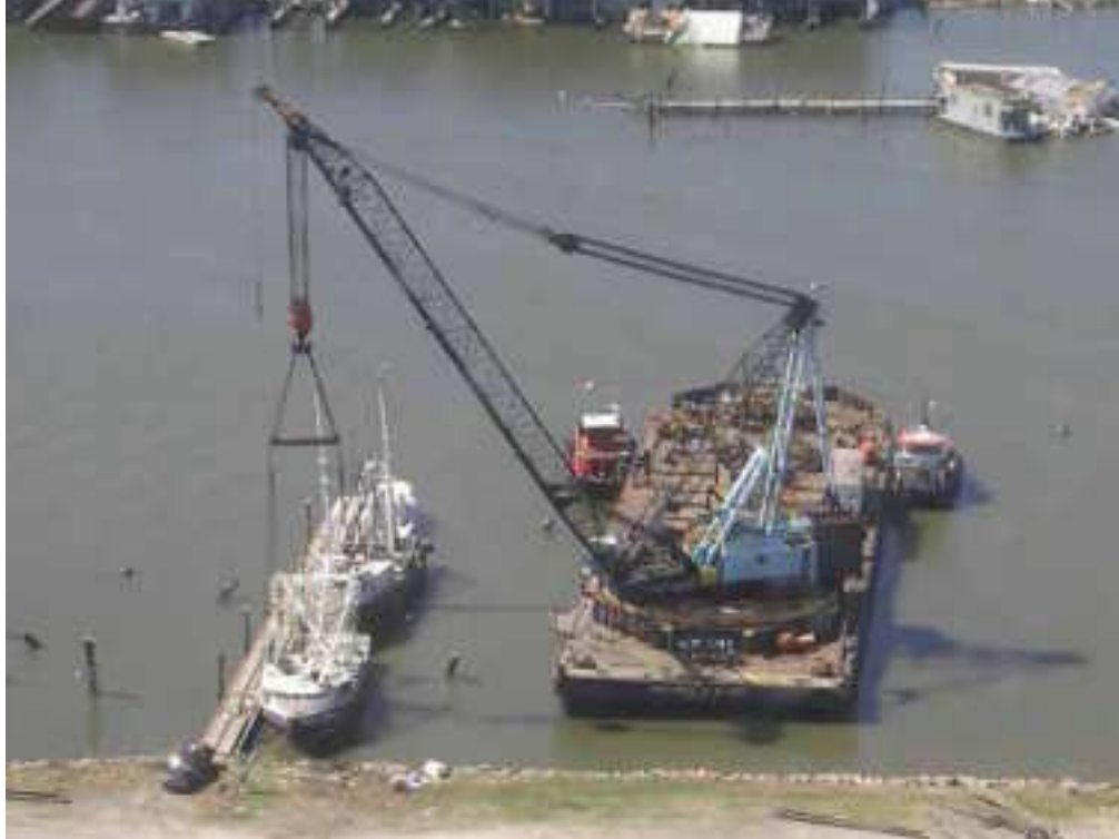
Figure 4-3. Donjon's Columbia New York refloating a fishing vessel in Venice, LA
