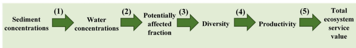
Fig. 1. Steps developed to assess the environmental impact of chemical mixtures in sediments on ecosystem services (ESs) of waterways. Step (1): Convert sediment concentrations into water concentrations. Step (2): Calculate the multi-substance potentially affected fraction msPAF(HC50) of aquatic species based on water concentrations. Step (3): Link msPAF(HC50) to diversity. Step (4): Identify the quantitative diversity-productivity relationship. Step (5): Update the correlation between productivity and the total value of ESs.
