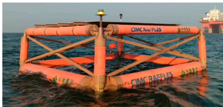
Figure 9. CIMC Raffles Offshore Technology Group's floating raft made from bamboo-based composite material. Reproduced with permission from authors [46].
