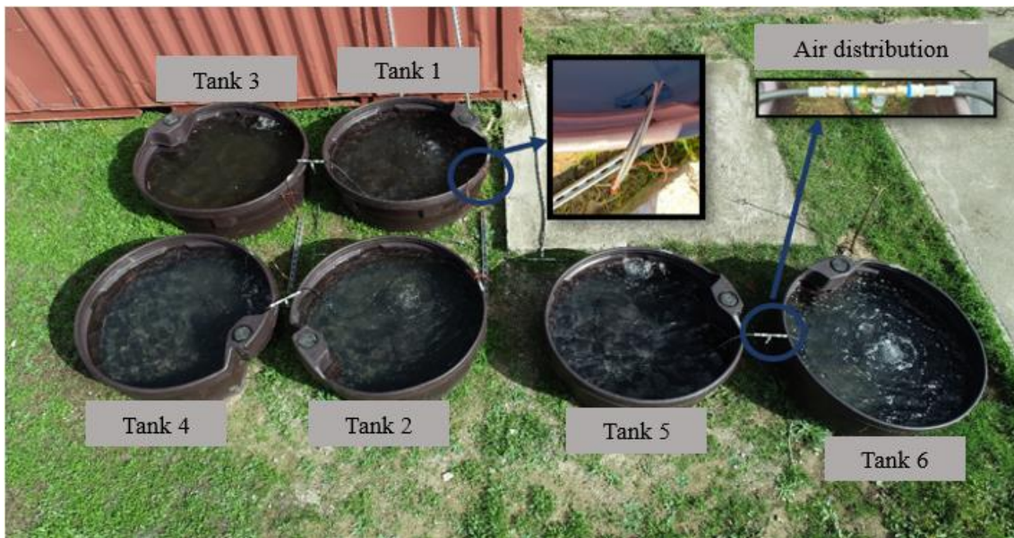
Figure 3: Experimental setup with the 6 water tanks. The air compressor and timer system are installed inside the red container (top of the image).
