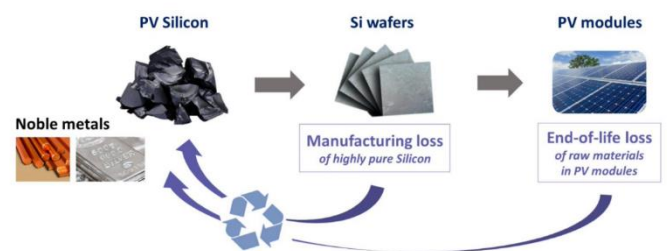
Fig. 1. Recuperation of ultra-pure silicon and other metals from solar panel's end of life Source: (ROSI – Return of Silicon, 2021)
