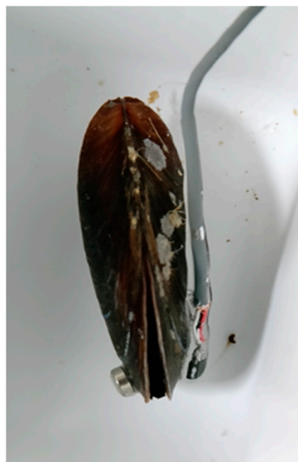
Figure 2. Valvometry sensor attached to the shell of a mussel in a lab setup: magnet (left valve) and Hall effect sensor (right valve).
