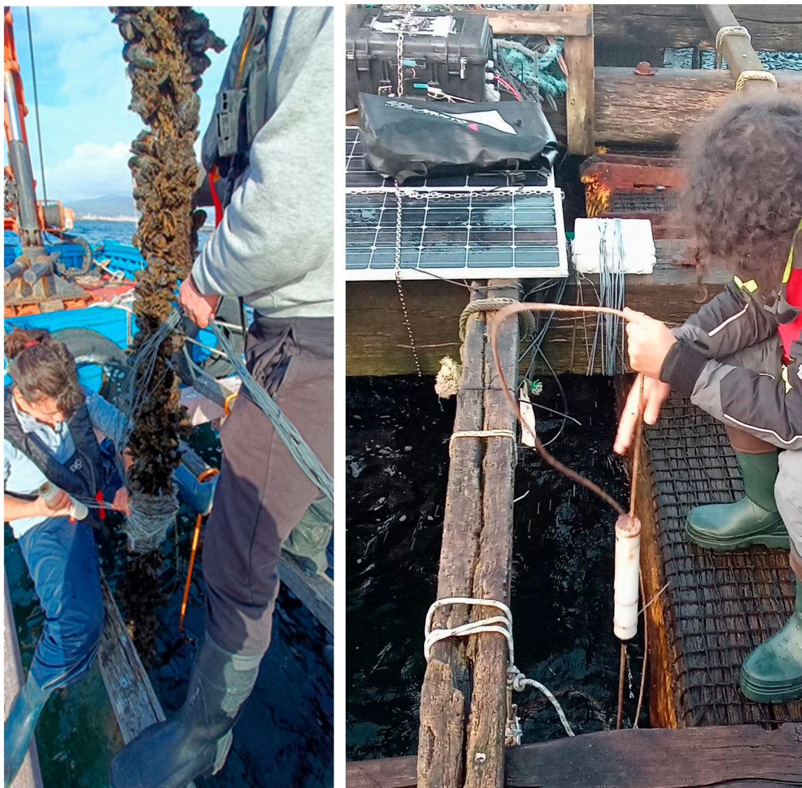
Figure 5. (Left): Operation of attaching the sensorised mussels to a rope of the raft; (Right): hydrophone deployment operation, the monitoring system integrated in the Peli case with the electronics can be seen in the upper left corner, behind the solar panels.
