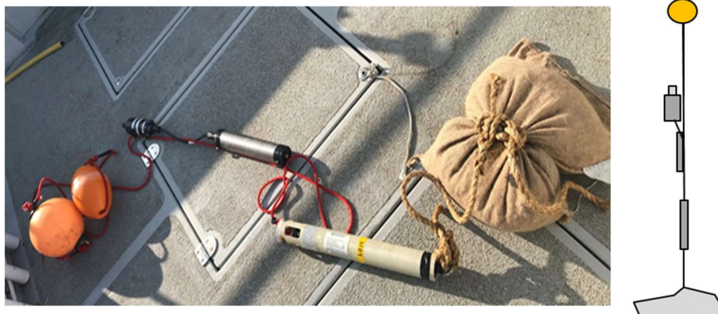
Figure 3. Photo and rig design of the hydrophone rig with a gravel bag as ballast weight, an acoustic releaser (light grey), a Soundtrap hydrophone system (black) with external battery pack and floatation buoys.
