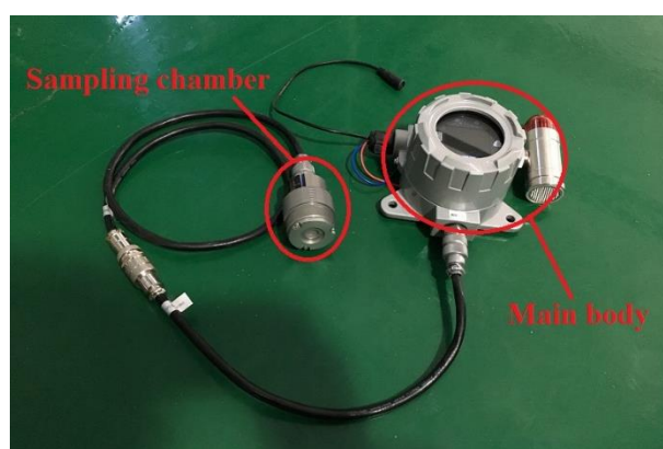
Figure 4. A fixed infrared gas detector with natural spread sampling mode.
