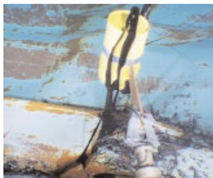
FIGURE P-1. ROV ATTEMPTING TO SAMPLE OIL LEAKING FROM PRESTIGE AT 3,500 M.
