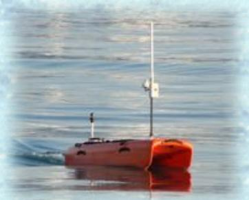
Data collection was mostly done at 0.7 – 1.3 m/s to reduce motion blur and the risk of air bubbles in camera's field of view.
