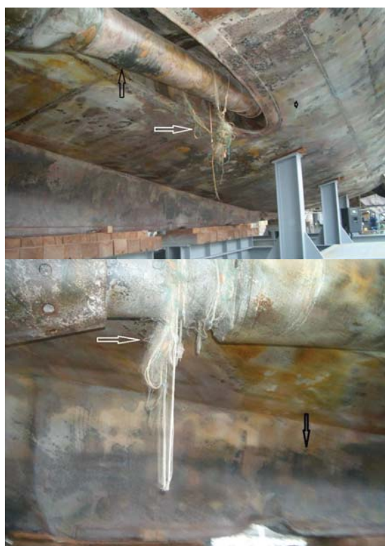
Figure 11: The tangled fishing net wires (white arrows) on the propeller axis indicate the running aground before the explosion, and the black charred hull surface (soot) may be due to the flame at the moment of the blast for an underwater explosion (black arrows). Also, it cannot be ruled out that the strong ICCP current might flow on the hull surface when it ran aground before the underwater explosion [2-3,5].
