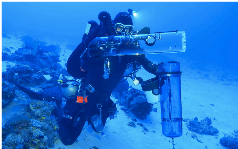
FIGURE 5 | A rebreather diver places the inner collection jar into the SubCAS, and then seals the chamber at an intermediate depth of ~60 m. The hinged access door, Velcro lock, submersible depth gauge and thermometer are visible on the inner collection jar, which is in the diver's right hand. The chamber cap and body are in the diver's left hand. In this version of the SubCAS, the valves and fittings on the chamber cap were protected by a white shroud constructed from an 18 cm diameter schedule 40 PVC cap.
