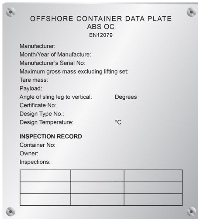
FIGURE 2 Template of Combined Data Plate and Inspection Plate
